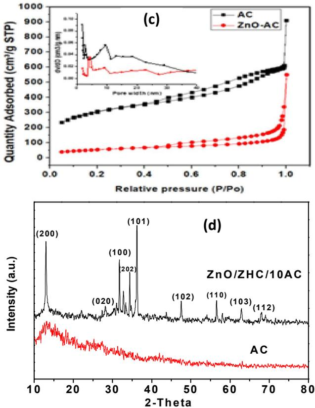
Figure 2. (a) and (b) SEM images of AC and ZnO/ZHC/10AC composite; (c) N<sub>2</sub> adsorption/desorption isotherms (inset: pore size distributions) of AC and ZnO/ZHC/10AC composite; (d) XRD patterns of AC and ZnO/ZHC/10AC composite.
