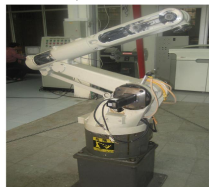
Figure 1. Six-link Almega 16 arm
